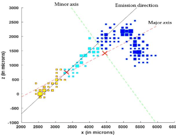
The figure shows the 2D binned image of a photoelectron track of a 9keV photon in Ne/DME 50/50 gas mixture at 200 torr pressure.
