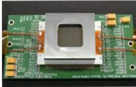
Sealed type MPGD and VLSI-ASIC
